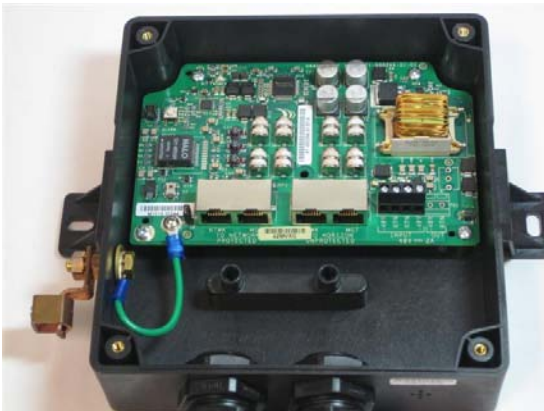
Figure 3-3 Outdoor Power injector/Lightning Arrestor
