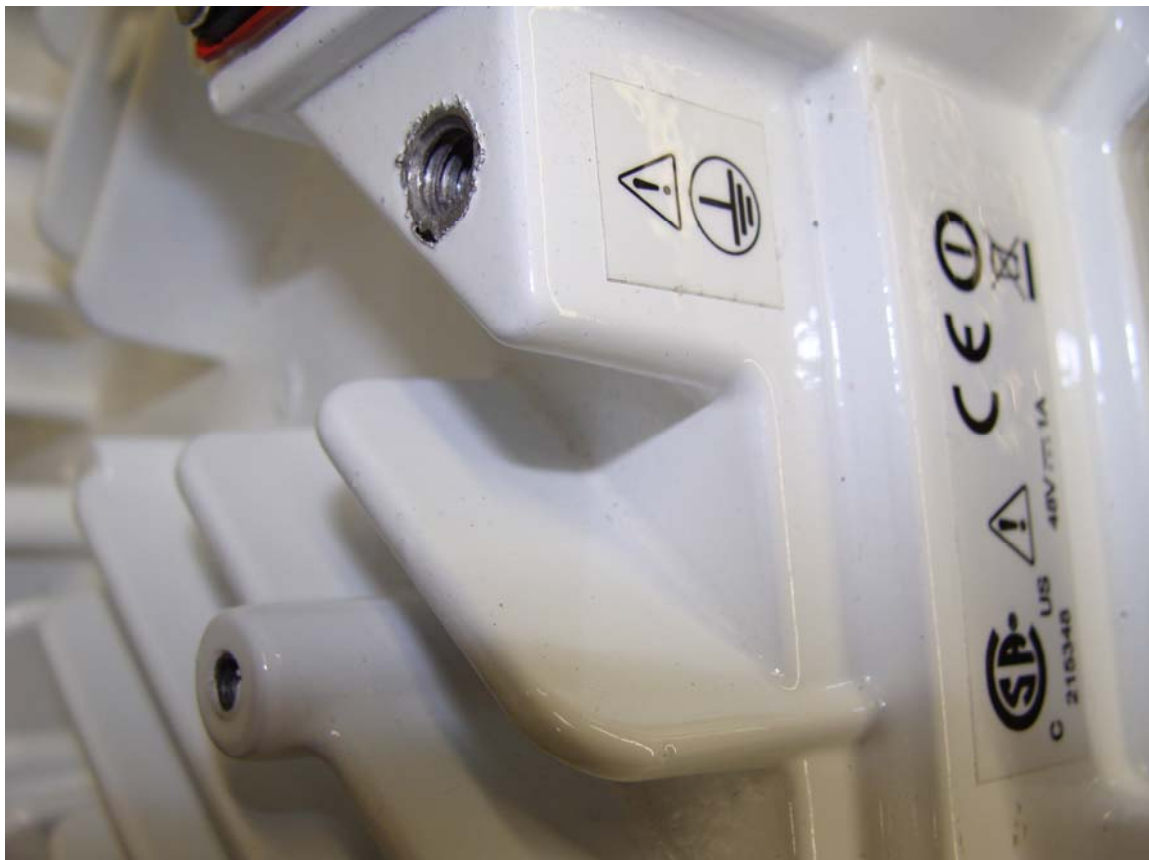
Close up Grounding terminal.
